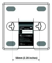
Figure 3-7: Measurement between Wall-Mount Slots
